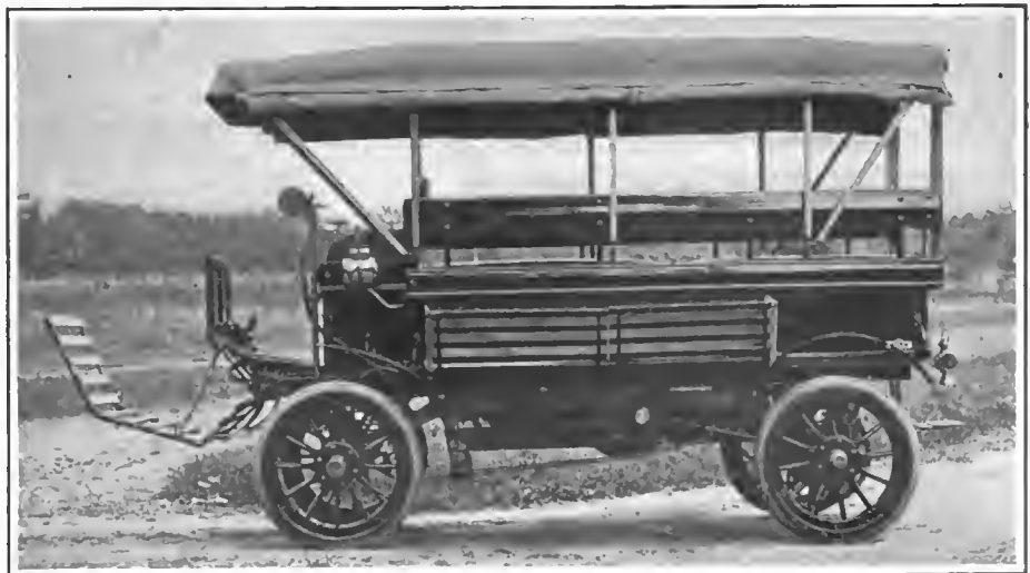
The colonial bus shown herewith has just been completed by the Knox Automobile Company and shipped to C. H. Martin, who is conducting an automobile stage service in Porto Rico. The bus has a regular double opposed Knox air-cooled motor. The special body seats fifteen passengers and has room in addition for baggage and mail. The car has a wheelbase of 96 inches and tread of 56 inches. The wheels are fitted with 4-inch solid rubber tires. There are two folding side racks that let down for carrying luggage and one that lets down in front for carrying mail pouches. The weight complete is 3,580 pounds. This vehicle can be converted into a patrol wagon by leaving off the racks. Orders for four similar busses for transferring passengers and baggage in Pittsburg have been placed by the Pittsburg Transfer Company.
